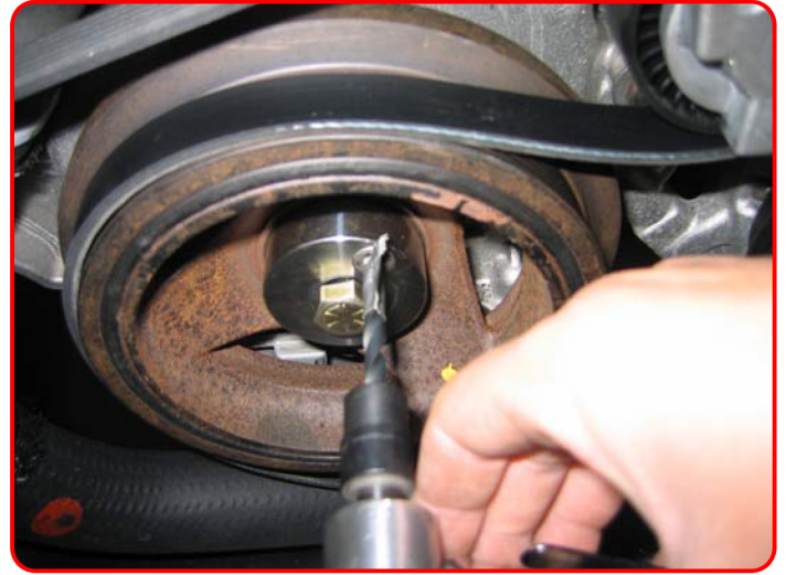
**Drilling pin hole in crank photo
