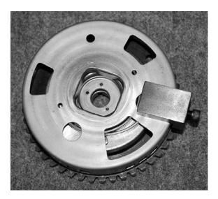
2. Turn the phaser over and loosen the circled bolt/pin that's opposite of the dowel pin slot, (in the picture below) one turn. Proceed to remove the remaining 4 bolts.
