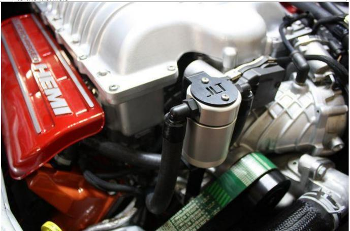
To properly clean the filter in the Oil Separator, spray any degreaser or solvent through it and let it air dry. Clean it every 10,000 miles.
