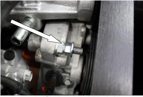
Use remaining nut to secure the JLT bracket to the stud. Using the 2 nuts you can "adjust" the position of the JLT bracket in and out.
