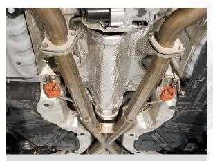
Detail 9: Inlets to X-pipe with hangers installed (shown with SW headers)
