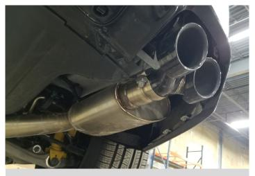
Detail 12: Right muffler assembly with tip installed
