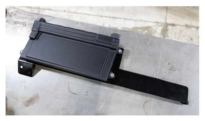
**3.** Then plug in the Gate-Way harness and factory connectors into the Gate-Way, then bolt the Gate-Way onto the factory ECU bracket.
