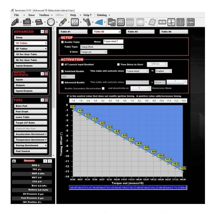
This advanced table needs to be used for torque management for transmission shifts.
