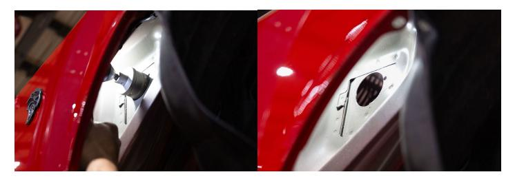
**3.** Once the hole is drilled, you can then run the Gate-Way harness up into the cowl from the inner fender.
