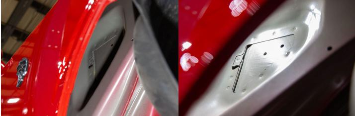
2. Start by drilling a small pilot hole in the center/top of the indent.
