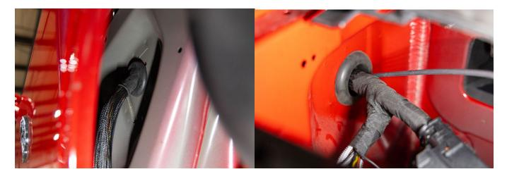
**4.** Now run the power harness under the car from the Holley ECU to the battery in the rear of the vehicle. There is a grommet in the trunk floor that it can be routed through.
