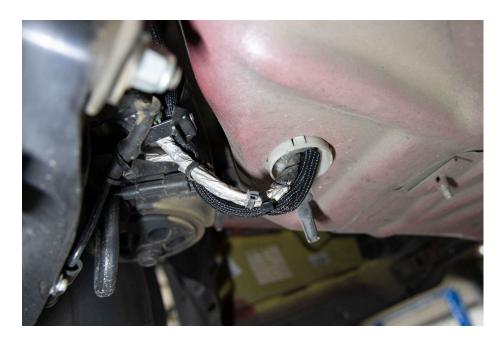
\*Note\* If using the Holley power harness (558-308), it will have to be extended about 6ft. We would also recommend adding a fuse to the harness near the battery. Custom power harnesses are available.
