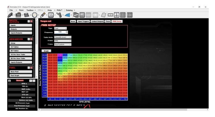
This table is the torque table that the TCM uses for torque calculations. The numbers represent newton meters, (0=-500NM, 500=0NM, 1000=500NM etc)
