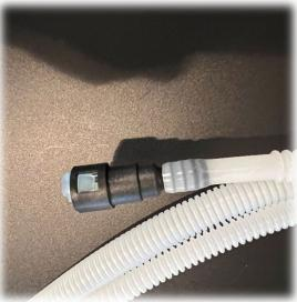
Note: It is important that the connector be fully seated in the hose as shown, failure to do so could result the failure of the connection and loss of fuel pressure.
