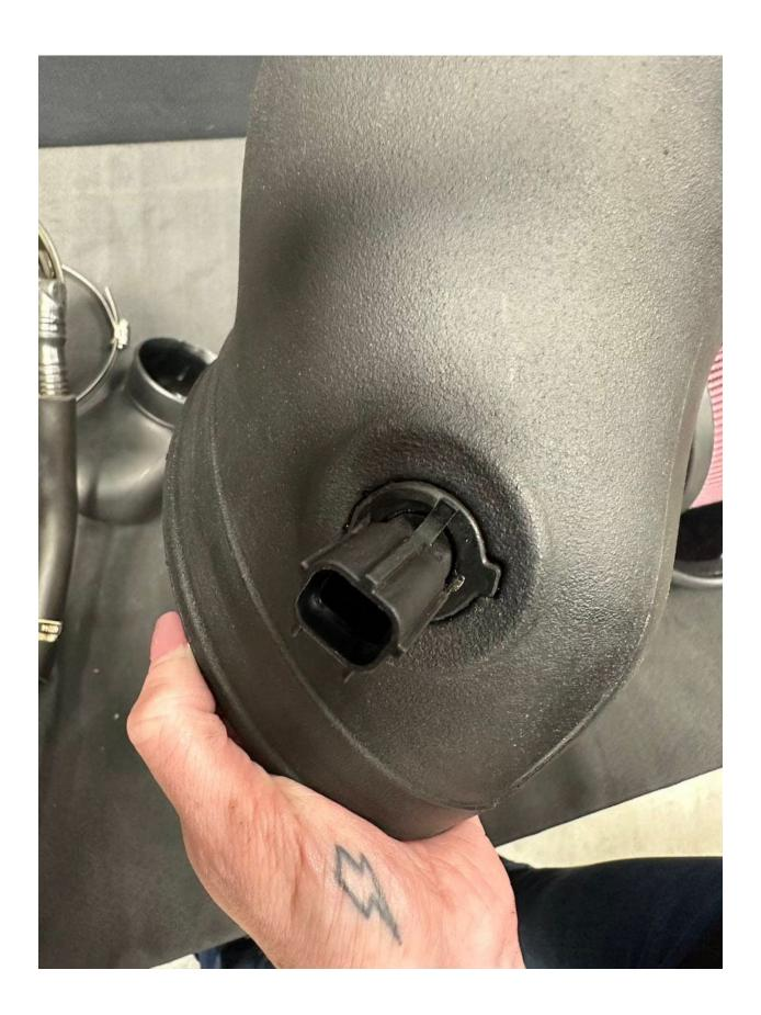
**Step 10**Install the Intake Tube into the filter then tighten down the hose clamps.
