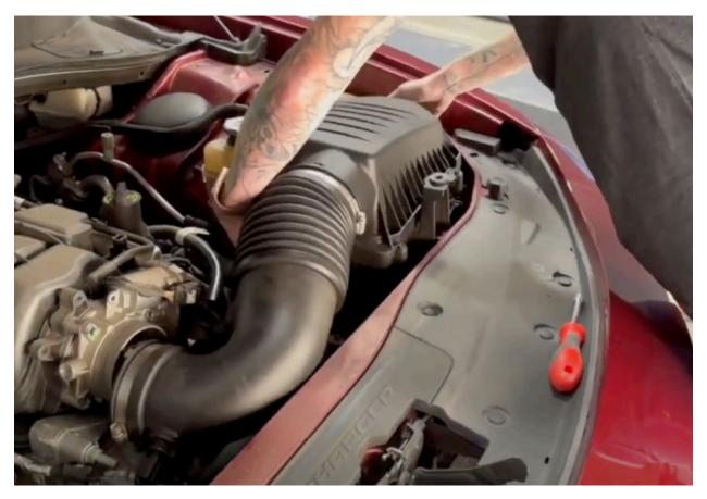
**Step 5**Install the filter into the JLT airbox.
