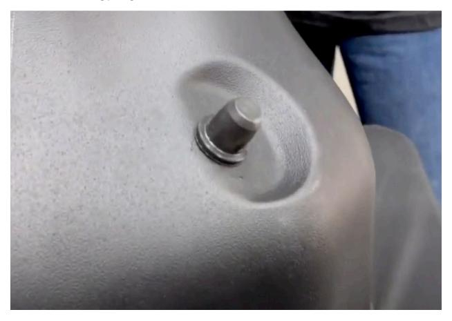
**Step 8**Install the grommet onto the JLT intake tube.
