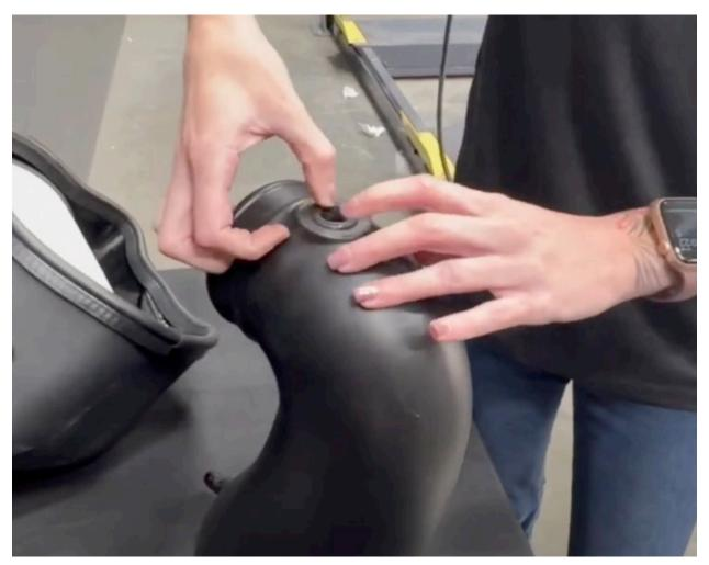
Care fully remove the IAT sensor from the stock tube. Then, install the IAT sensor into the JLT tube by twisting it so the tab is as shown.
