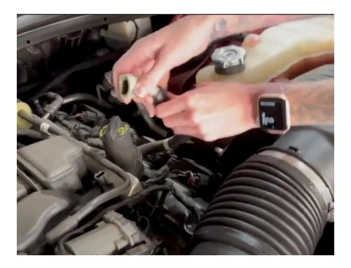
**Step 4**Remove the stock intake from the vehicle.
