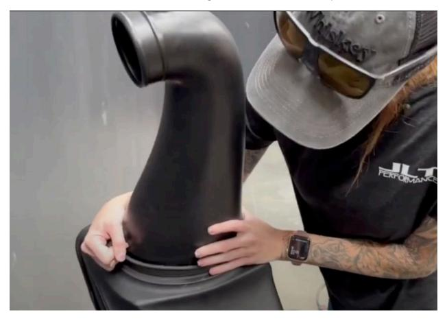
If your Challenger has a functional headlight scoop, install the seal and scoop onto the airbox. Make sure the arrows on the coupler line up as shown in the picture. Widebodies use the shorter scoop, and narrow bodies use the longer scoop.
