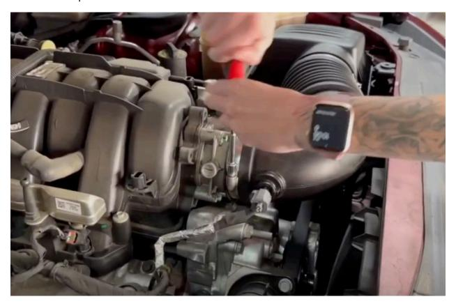
Disconnect the quick connect fitting or the hose (depending on the specific vehicle you have) from the airbox. If you have a quick connect fitting, then remove the fitting from the hose.
