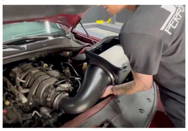
**Step 14**Once the intake is in place, reinstall the stock screw and tighten down.
