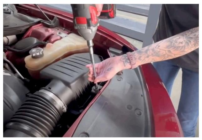
Remove the engine cover in order to gain access to the hose clamp and IAT sensor. Loosen the hose clamp and disconnect the IAT sensor.
