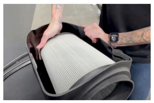
**Step 6**Install the edge trim on both the top and bottom of the airbox.
