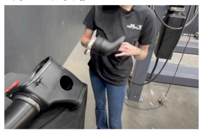
**Step 12**Install the Intake into the vehicle by fitting the mounting grommet into place on the vehicle and sliding the coupler over the throttle body.
