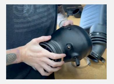
Pushing the coupler as far as possible onto the tube makes installation easier. Install the intake tube and tighten down the hose clamps.
