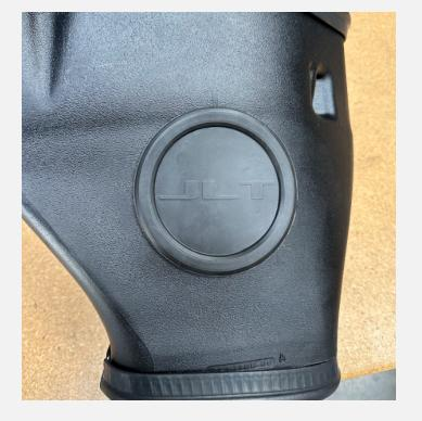
Install the grommet onto the bottom of the airbox.
